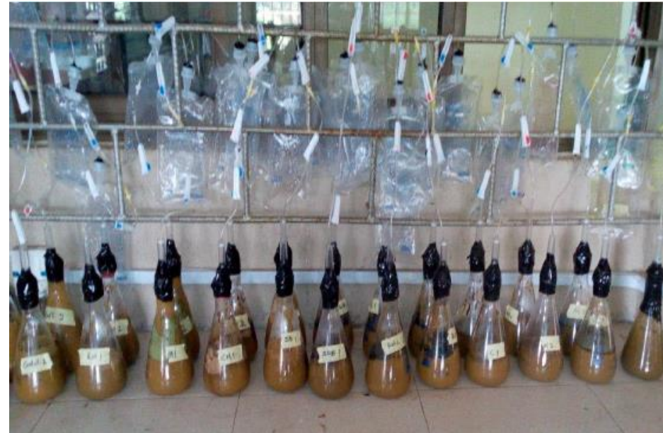
EFFICIENCY OF BASIC ADDITIVES ON H_2S REMOVAL
